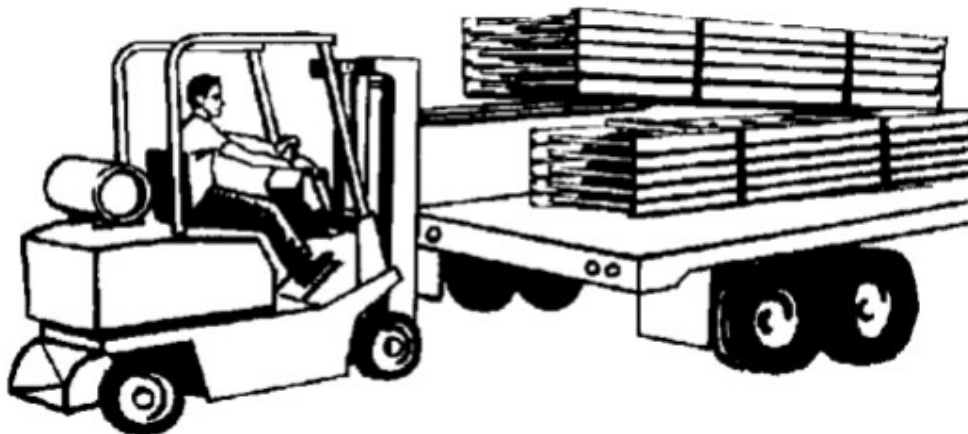
Figure 1-2 Not Correct—Except when Using Extended Forks for Skidded Bundles
